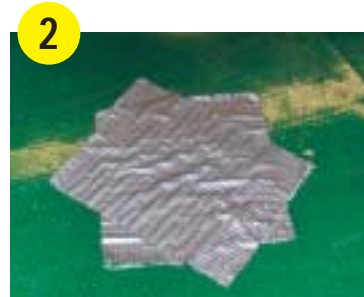
2 Duct tape may work in an emergency. But it is ugly and water can still leak into the foam core of the board.
