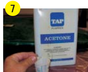
7 Remove a piece of the foam core and place in Acetone. If nothing happens, use Surfboard Resin for repair. If foam dissolves, use epoxy.
