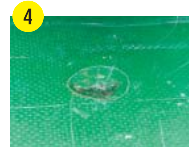
4 With the ding exposed, it is easy to see how much of the fiberglass skin must be removed for the repair.
