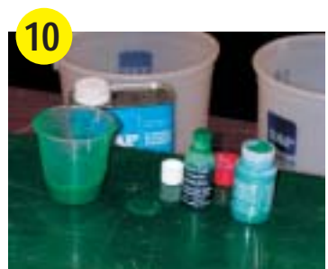
10 For small dings, resin without glass can be used for repair. If you do not plan to paint the board, use pigment and dye to color match the resin. Fill balance of hole to slightly above the surface.
