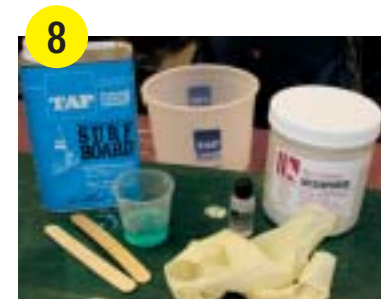
8 Assemble the materials you will need – mix Microspheres and Surfboard Resin to make a resin foam to fill the hole.
